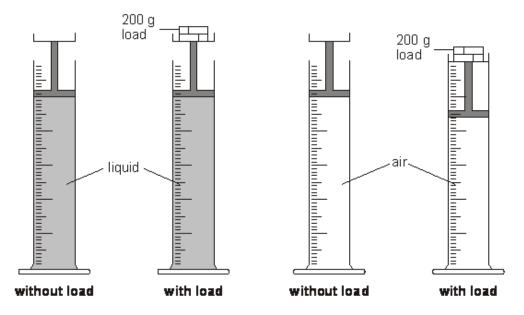
(i) When the loads were added to the pistons, the volume of the liquid did **not** change but the volume of the air decreased.
