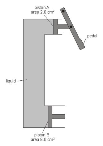
At each end of the container there is a piston. Piston A has a smaller area than piston B.
